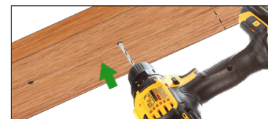
Figure E. (LEFT) Mark the pre-drilled screw holes in the channel to the underside of the top rail.
