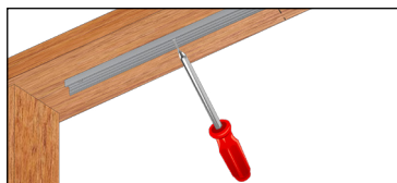
Figure G. (LEFT) Use a Phillips head screwdriver and screw in the channel to the underside of the top rail.
