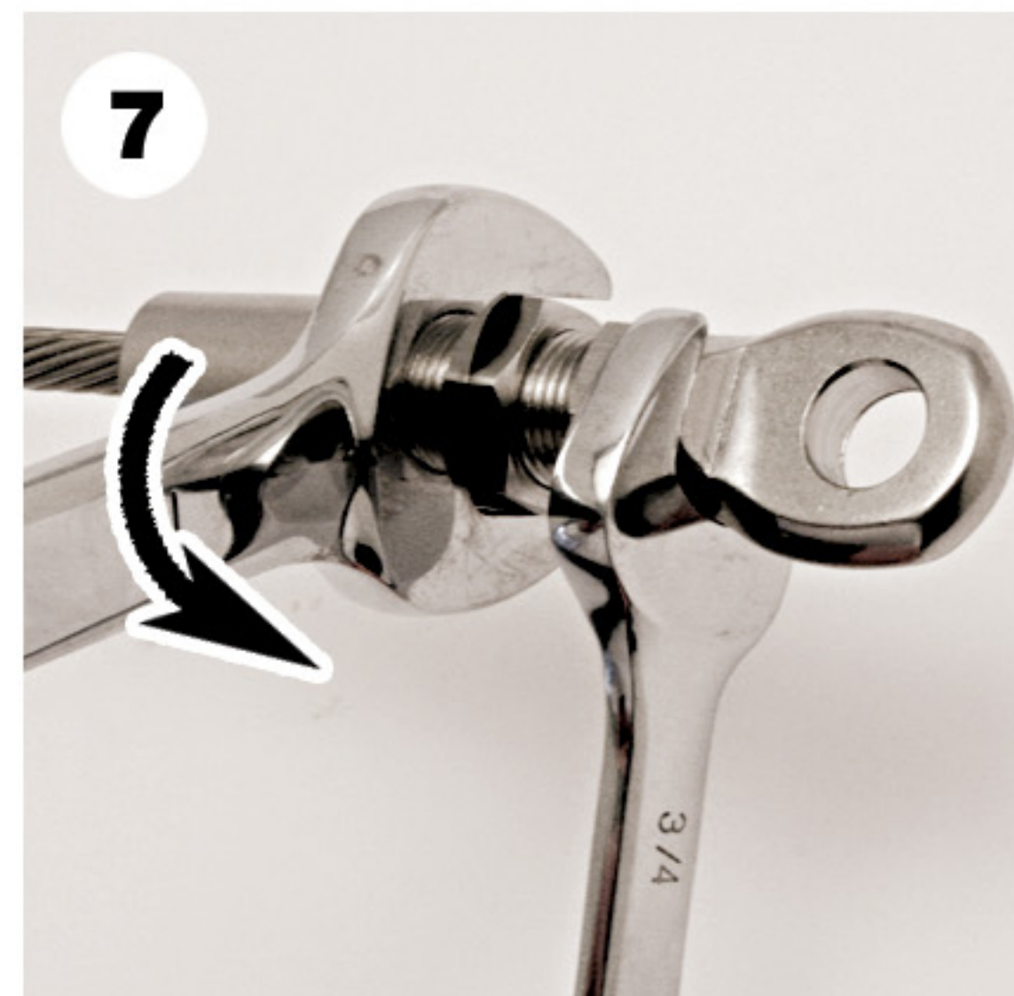
7. Using wrenches tighten the Cone onto the head as far as possible.
